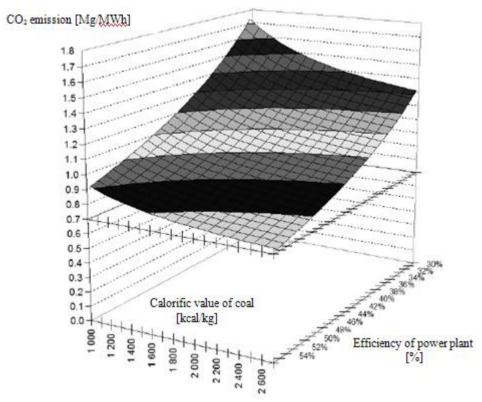
Fig. 3. Dependency of CO<sub>2</sub> emissions from power plant efficiency and calorific value of lignite (Jurdziak and Kawalec, 2010)
